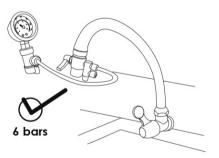
Please ensure that the maximum water pressure does not exceed 6 bars to avoid severe damage to the membrane filter. If the water pressure is lower than 2 bars, installation of a water pump is recommended.
