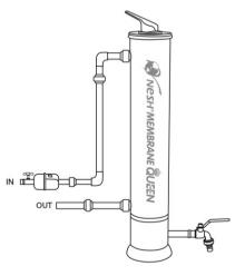
Before the usage of a newly installed product, please ensure you flush away the protective layer on the membrane filter for approximately 30 minutes until all traces of foamy substance are replaced with clear water.
