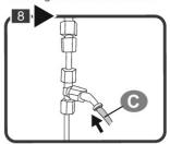
Insert silicone tube C into the T-Connector
