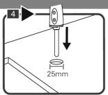
Install the faucet. Please ensure that the diameter of the hole for installing the faucet is 25mm.
