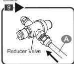
Insert white tube A into the reducer valve
