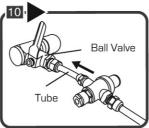
Connect the reducer valve to the ball valve.
