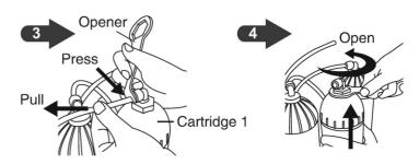
Use the opener to press on the button elbow of the Cartridge 1 and pull out the white tube.
