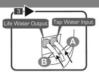
Insert white tube A to the right. Insert white tube B to the left.
