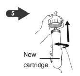
Hold firmly onto the new cartridge and tighten.
