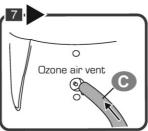
Insert silicone tube C into the ozone air vent.
