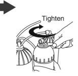
Place the ceramic filter back into the cartridge and tighten the base cover. Make sure the O-Ring is placed at the correct position.
