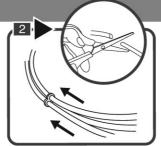
Cut the white tube into required length. Then tie the white tubes and silicone tube together using the 3-way hose ring.
