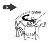
Place the ceramic filter back into the cartridge and tighten the base cover. Make sure the O-Ring is placed at the correct position.
