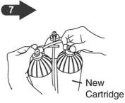
Insert the white tube back into the button elbow of the cartridge.
