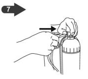
Insert the white tube back into the button elbow of Cartridge 1.
