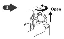
Twist and open the top cover. Pull out the ceramic filter
