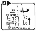
Once all tubes are fixed, attach the diverter valve to the tap & tighten
