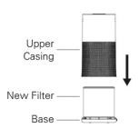
Lock the Filter Lock by sliding it to the right until you hear a "click" sound. Plug in and turn on the product.
