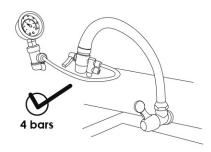
Please ensure that the maximum water pressure does not exceed 4 bars to avoid severe damage to the membrane filter. If the water pressure is lower than 2 bars, installation of a water pump is recommended.
