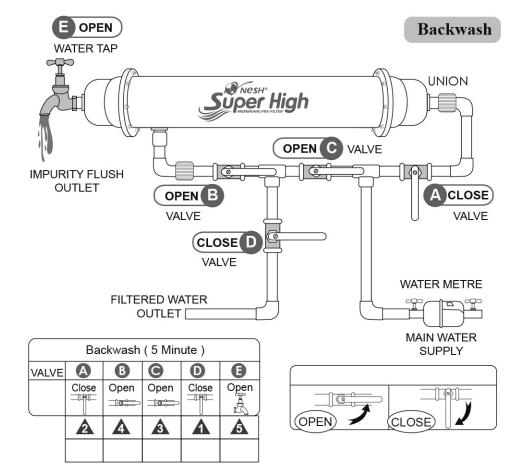
Note: After BACKWASH, proceed to Special FLUSHING (see diagram at page 7)
