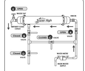
Before the usage of a newly installed product, please ensure you flush away the protective layer on the membrane filter for approximately 30 minutes until all traces of foamy substance are replaced with clear water.
