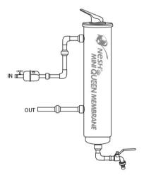
Before the usage of a newly installed product, please ensure you flush away the protective layer on the membrane filter for approximately 30 minutes until all traces of foamy substance are replaced with clear water.
