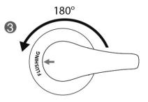
After backwash, turn 180<sup>o</sup> back to "Flushing".
